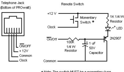
\* Note: The switch MUST be a momentary type. If no LED status display is required, using the switch to short +12V and the Clock will toggle the unit on and off.
